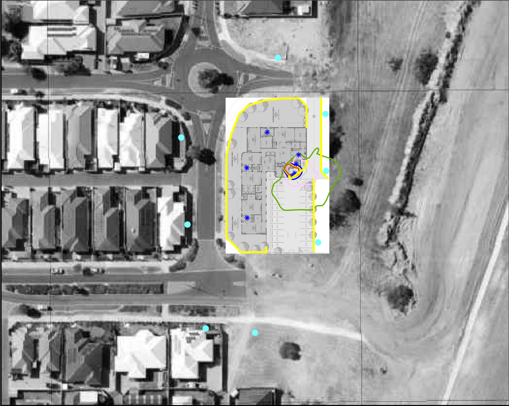
Figure 4-2 Mechanical Plant Noise Contour Plot (1.4m AGL), dB LA10
