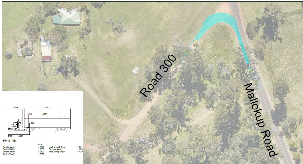
Figure 10- Swept Path inbound direction for 19.0m truck
