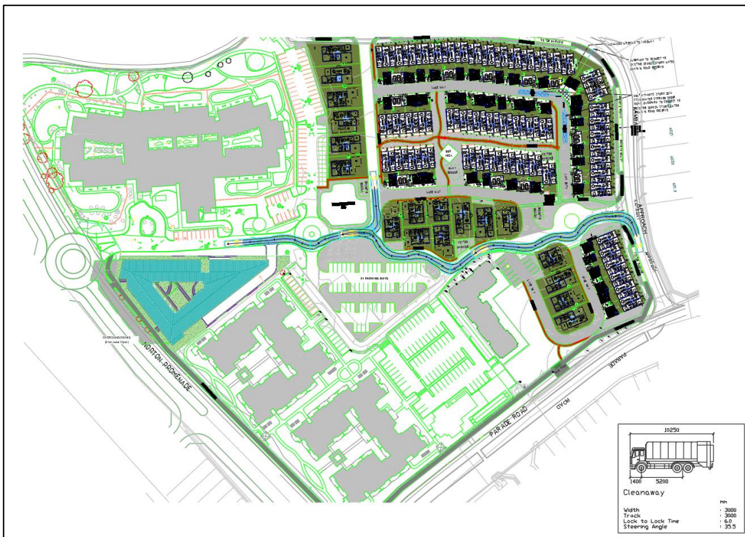
Figure 2-4 Swept Path – Waste Collection
