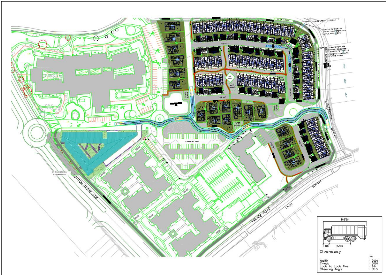
Figure 5-3 Swept Path – Waste Collection
