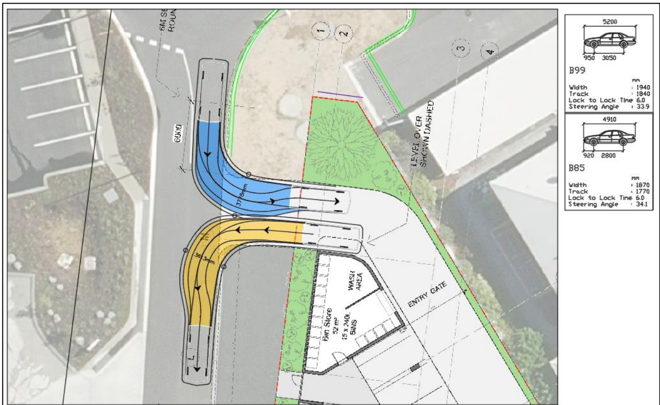
Figure 6-1 Swept Path – Access
