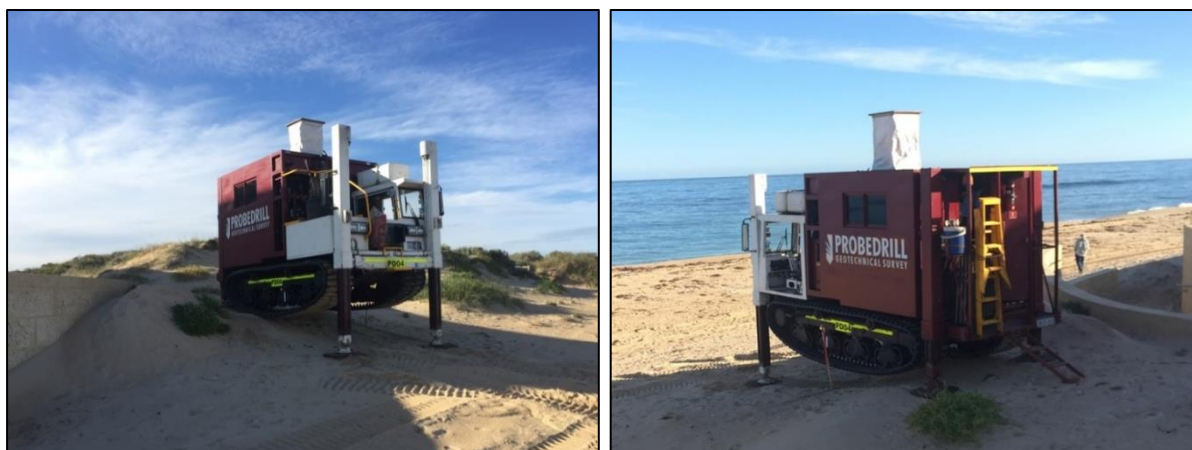
Figure 7: CPT data acquisition during a previous coastal investigation.
