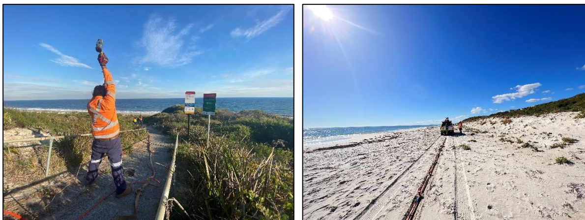
Figure 3: MASW data acquisition using a seismic streamer.
