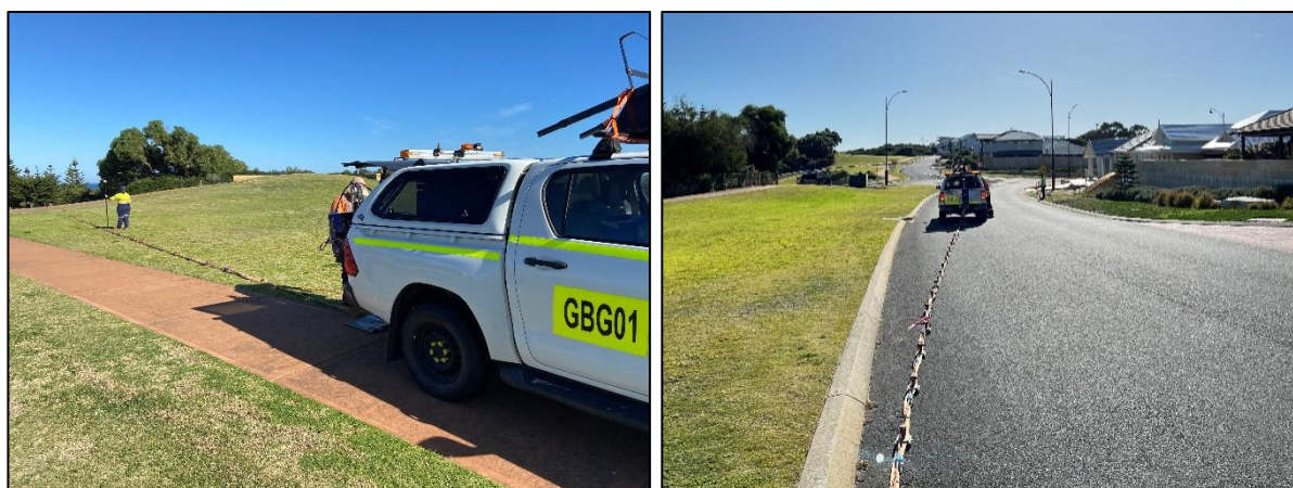
Figure 3: MASW data acquisition using a seismic streamer.
