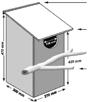
The top edge of the roof should be weather sealed with a folded strip of sheetmetal, aluminium angle or a rubber flap. (An old rubber inner tube is OK)
